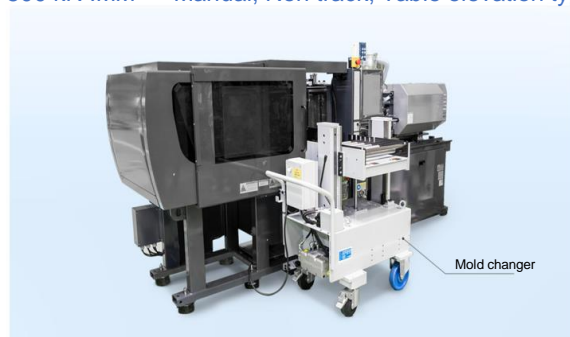
500 kN IMM — Manual, Non track, Table elevation type
