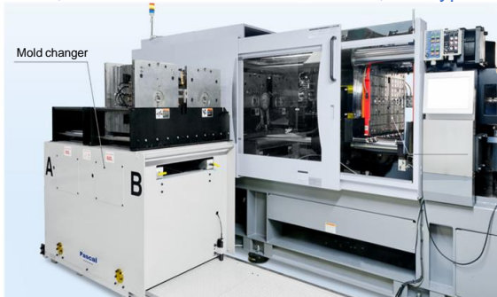
500 kN IMM — Manual, Rail type
