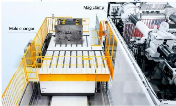
2,500 kN Two-color IMM — Manual, Rail type
